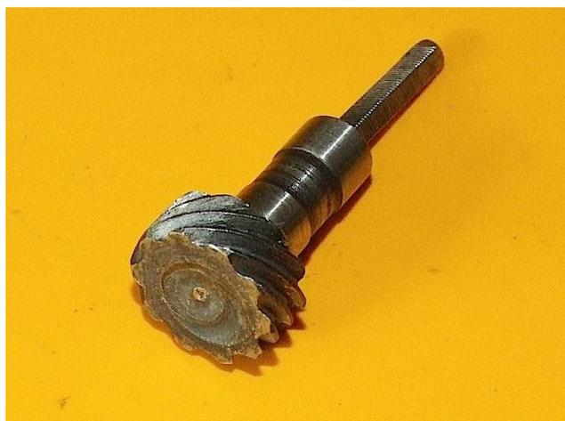
The gear-teeth get worse on the drives from the far-east. The teeth on this one have not been machine cut, they are just as they left the mould, when this item was cast. This one has had the ferrule knocked out also, you can see that there was no weld-penetration, just a surface mark where the weld was “stuck-on”.
