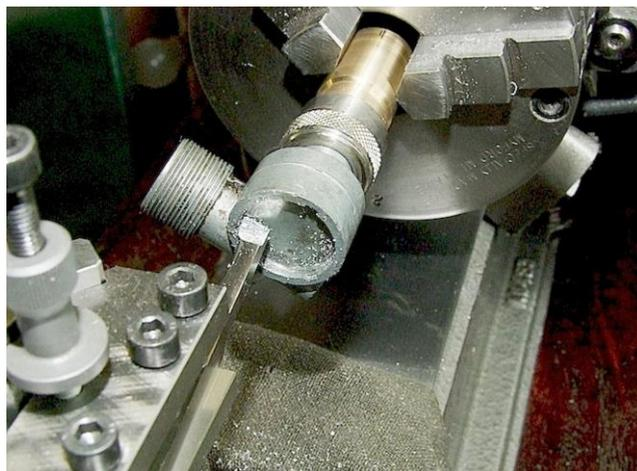
Doing this allows me to open the drive quickly, and cut a groove for a circlip to hold it together again, all in one operation. I do the same thing to get at the spiral-gear.
