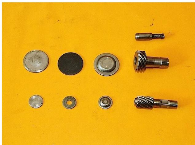
You can see the broken wire-stub, which I have knocked out of the big bevel-gear, the spiral-gear, the thrust-face and the packing shims that set the end-float.
