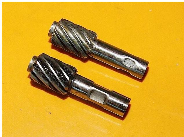
The top pinion came from a drive that refused to operate the speedo reliably. These pinions pick-up on the squared end of the speedo-cable. But they don't have a square hole. Not even the Smiths ones do.
