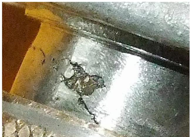
Here is another that has suffered abuse to its stem. In this case it has come undone from the transmission and has been running loose and rubbing on something. Again you can see how thin these are:
