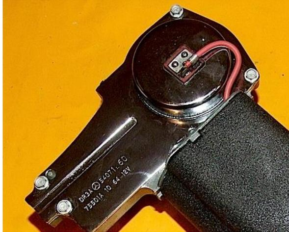
The head-size is **4BA** and the best tool is a nut-driver or a small socket, spanners are fiddly.
