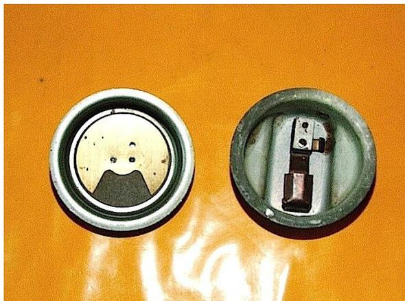
The parker is wired to one of the motor connections by the obvious red-wire that you see on the cap. The parker connects the **red-wire** to the **body** of the motor.
