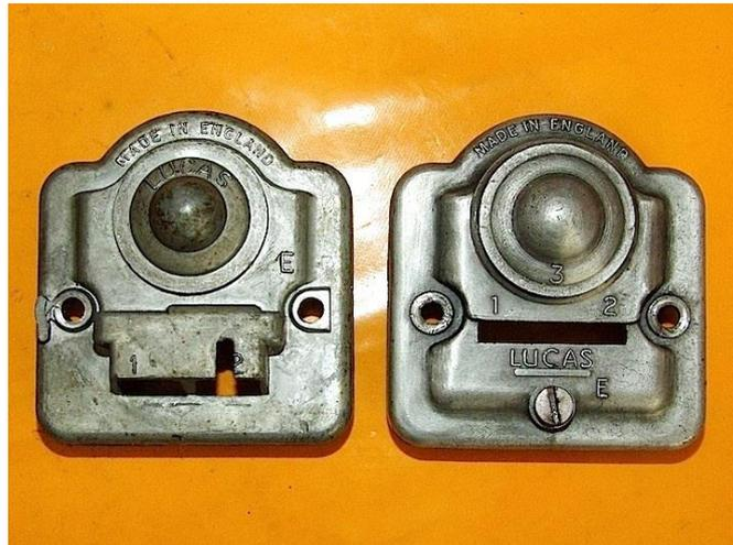
But two-speed motors need three connections. These motors have a “flying-lead” with three wires in it. These wires have “bullet” terminals on the ends.
