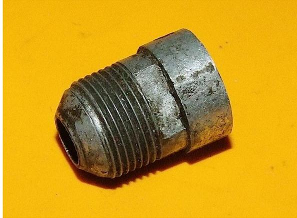
If you ever encounter a nut that is stuck onto it's nipple, **DO NOT** be tempted to use the motor gear-case as a kind of spanner to undo it. All that will happen is that you **will split** the gear-case.
