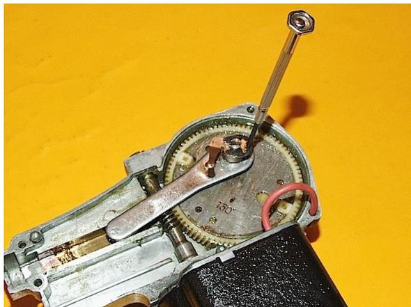
Take off the parker-contact and lift up the crank-arm. There may be a **small washer** that comes free when you do this. Look after it and note where to refit it, between the arm and the gear-wheel.
