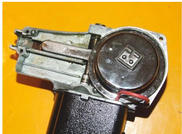
The crank-pin stops near to the small “pip” knocked into the cap. The purpose of this pip is to help you set the self-parker.
